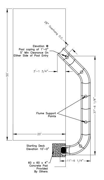
\*Elevations Based On A Pool Deck @ 0'-0"
